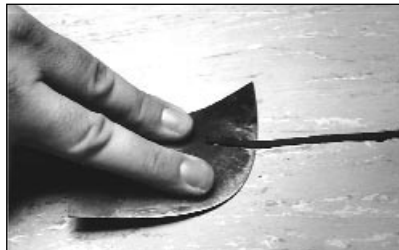
Figure 10: Second pass finish trimming.
