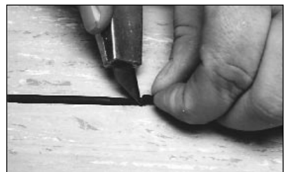
Figure 5: Trimming excess thread.
