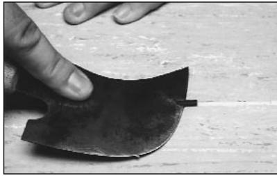
Figure 6: Trimming for weld splice.
