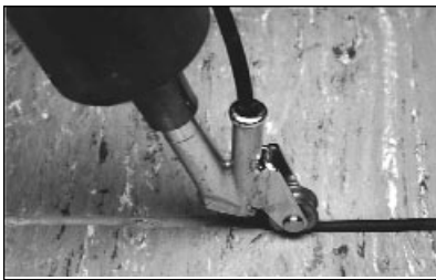
Figure 4: Proper welding angle.
